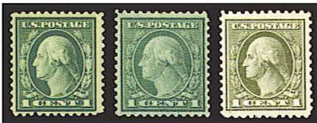
Figure 17. Use of 3 printing presses. 1¢ stamps Scott #498, #545 and #525, examples of stamps printed by intaglio flat plate press, intaglio rotary press and offset lithographic press, respectively. Each type of press produced stamps of differing heights and widths, and differing ratios of these dimensions. In addition, slightly different perforations were applied to flat and offset press products than were used on rotary press issues.
