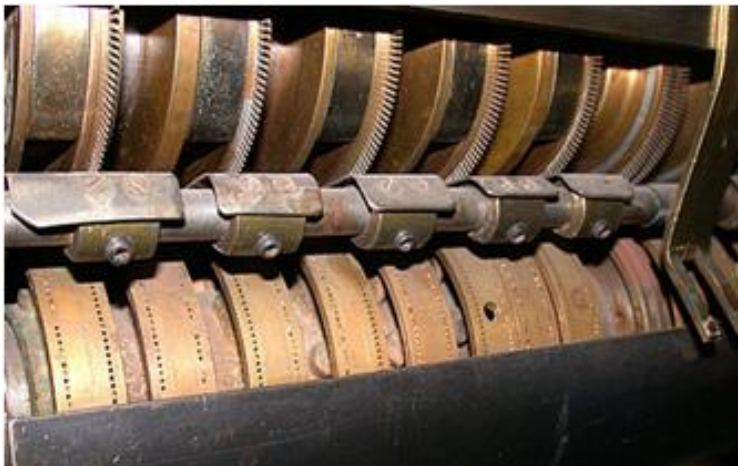
Close-up of SI NPM machine, showing matching sets of pins & holes (ca. 1913)
