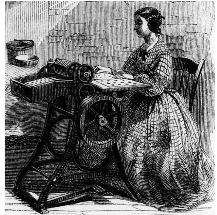
Rotary Perforating Machine (ca. 1861)
