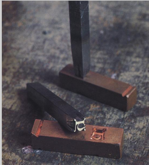
1. Steel punch strikes letter into copper blank (matrices).
